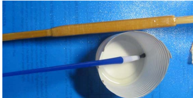
Picture 16 Coat the ferrule (and the sections) with varnish.
