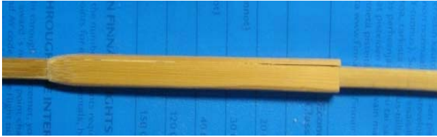
Picture 13 The ferrule is sanded and ready to be wrapped.
