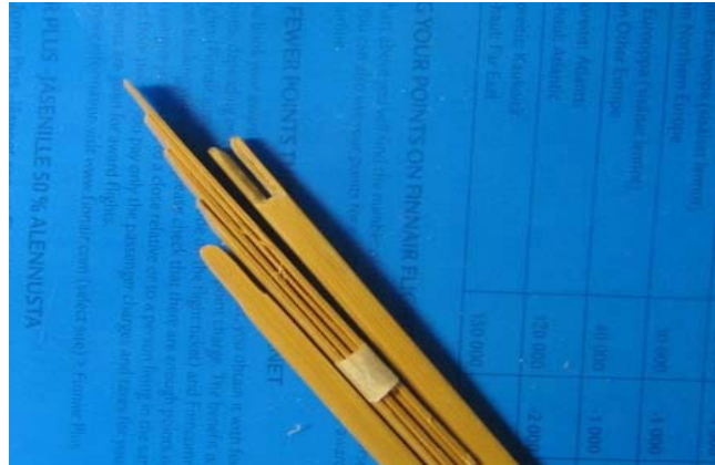
Picture 7 The ferrule strips are sanded thin at the tip end.
