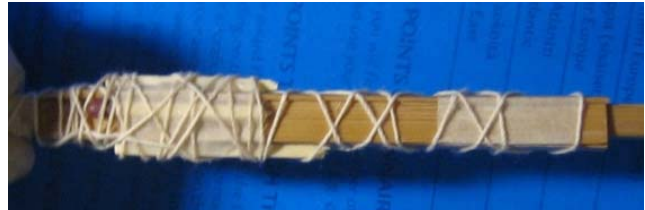
Picture 11 The ferrule is glued and wrapped. Here the tip section is on left side (with glue) and butt section (no glue) is on the right side.
