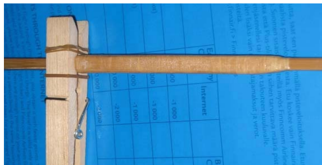
Picture 16 Clothespin tool to loosen a jammed ferrule.
