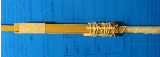
Picture 9 The construction of the ferrule.
