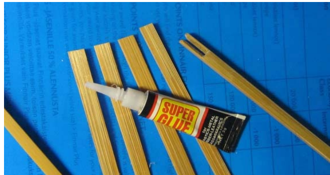
Picture 8 The surface of the ferrule components are coated with cyanoacrylate glue.
