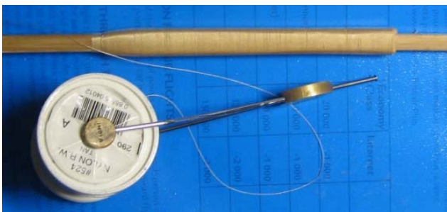
Picture 14 The ferrule is wrapped using the same kind of thread as the guide wrappings.
