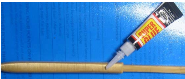
Picture 15 The wrapping is finished with varnish or cyanoglue.
