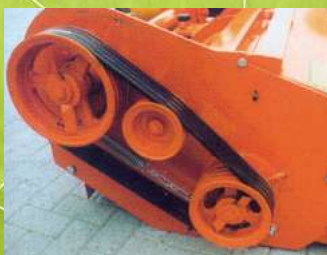
V-belt drive with automatic belt tensioner
